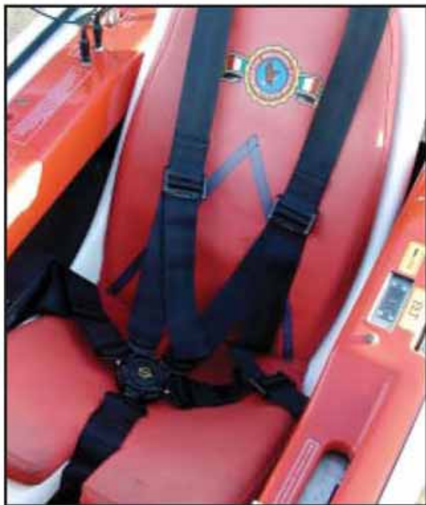
FIVE WAY – The Sky Arrow I flew had this excellent five-point restraint system, where some Sky Arrows have only shoulder and crotch belts. The company feels this is adequate but some feel otherwise.
