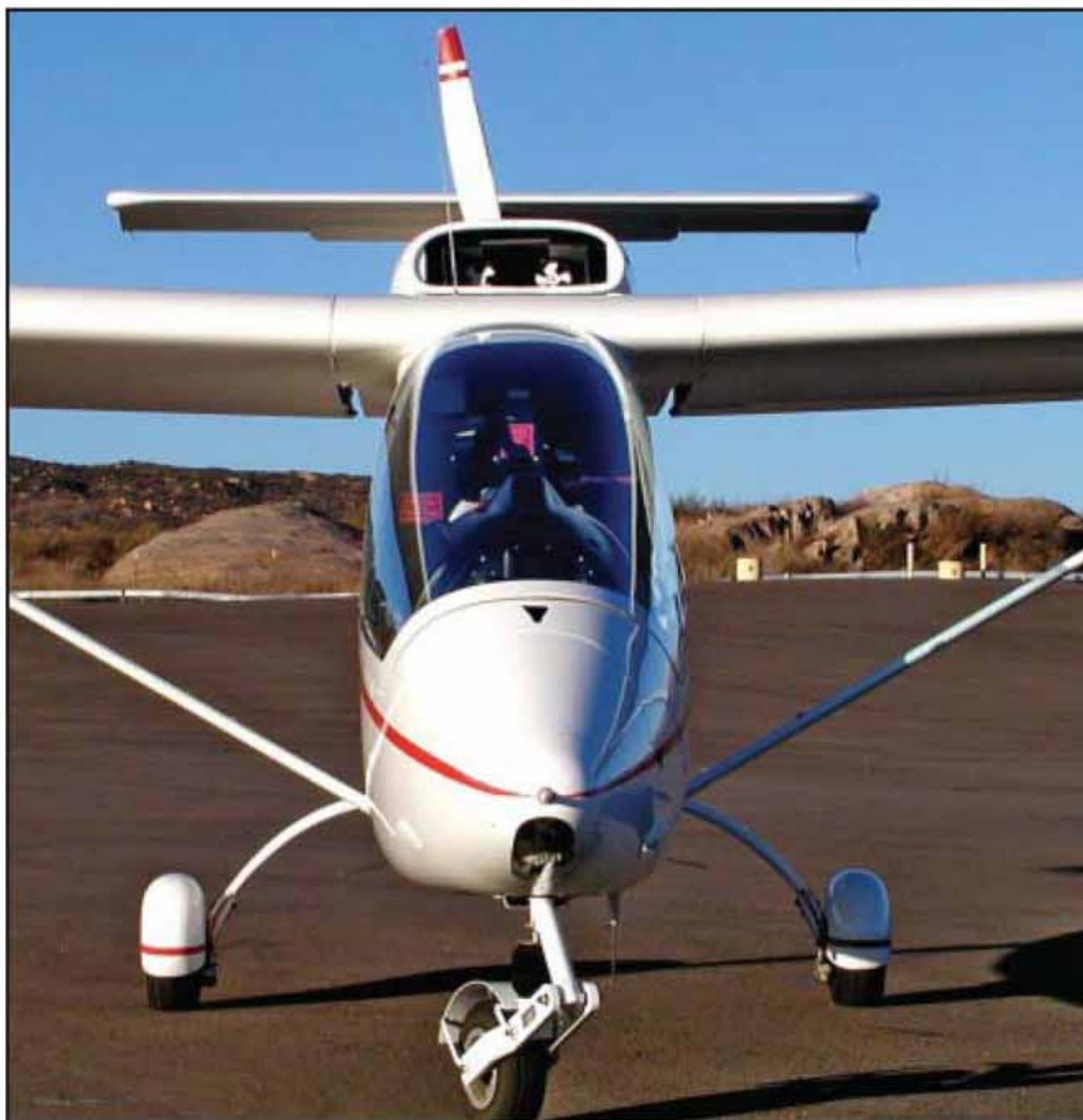
LEAN TANDEM – An advantage of tandem design is that the fuselage is lean with low drag compared to side-by-side designs. The rear seat is elevated to give better visibility.
