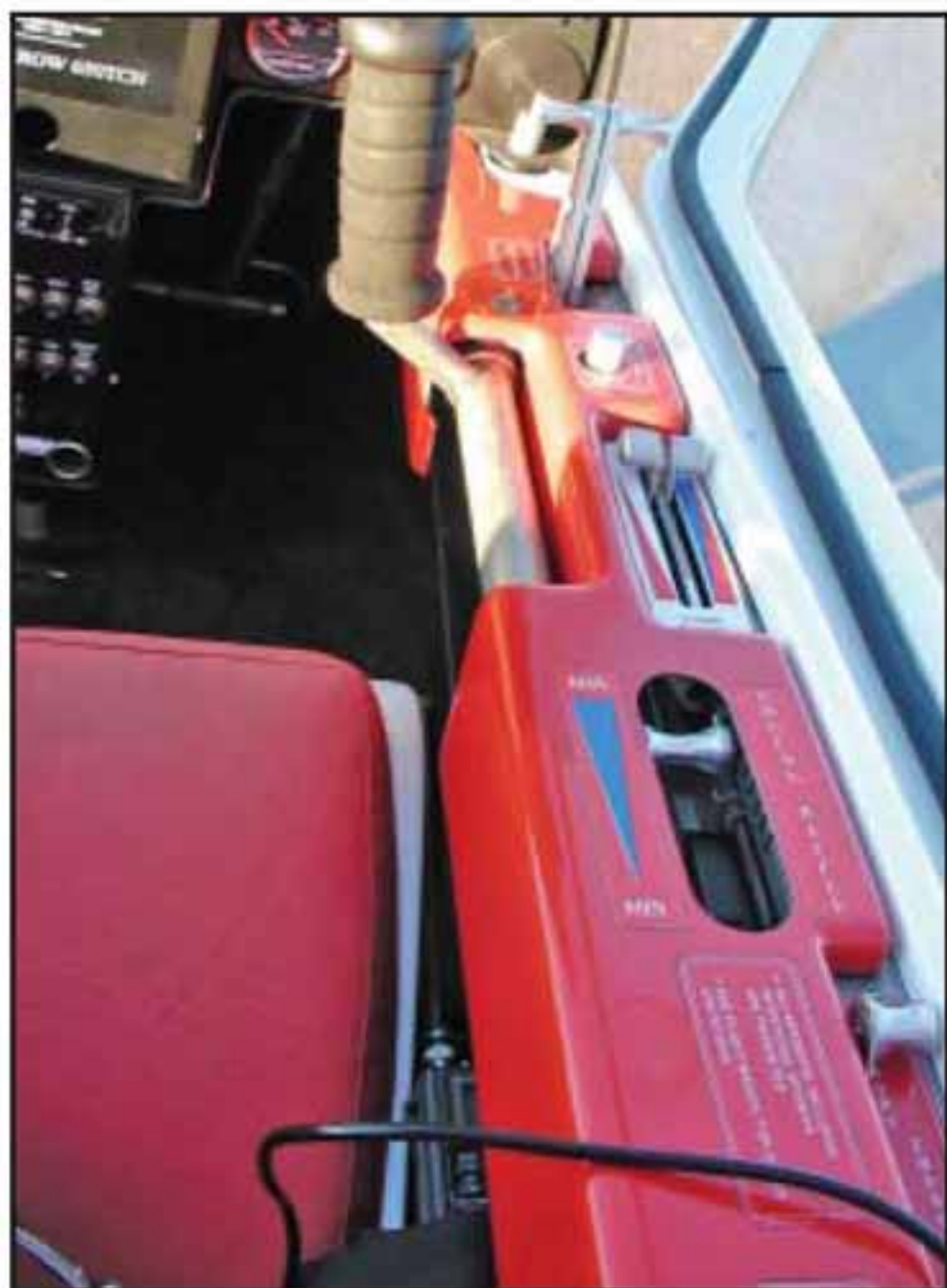
Top Photo: LEFT SIDE – On the left side of the pilot are controls to open the canopy, adjust carburetor heat, trim, choke, ignition switch, and fuel shutoff.
