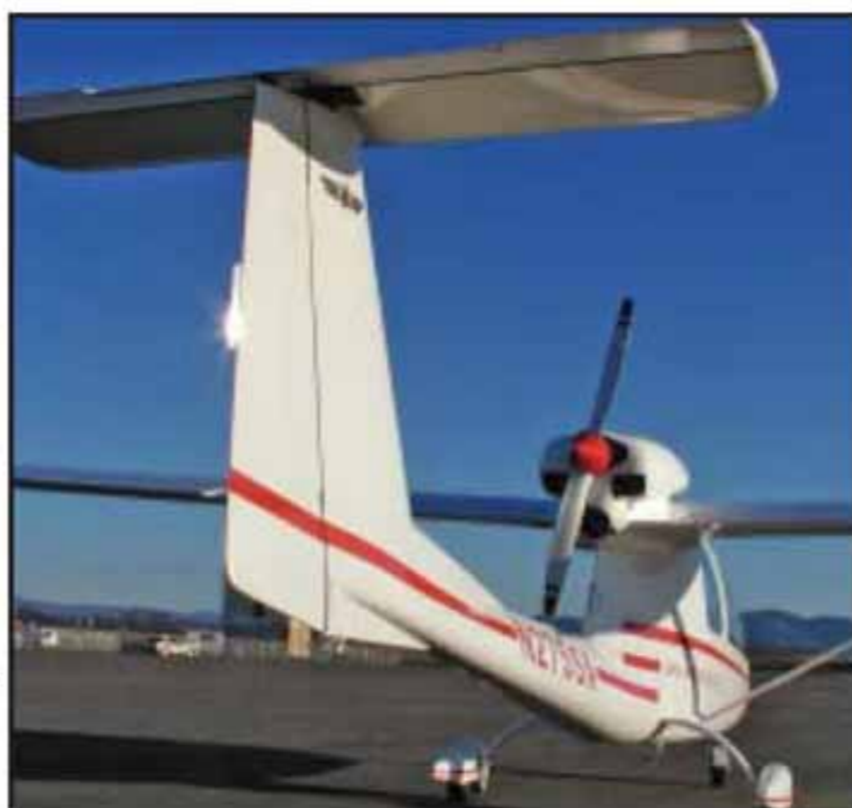
TEE TAIL - The high tail of the Sky Arrow follows modern design that favors the T-tail look. It's out of reach but you can lower the plane by the tail for inspection.
