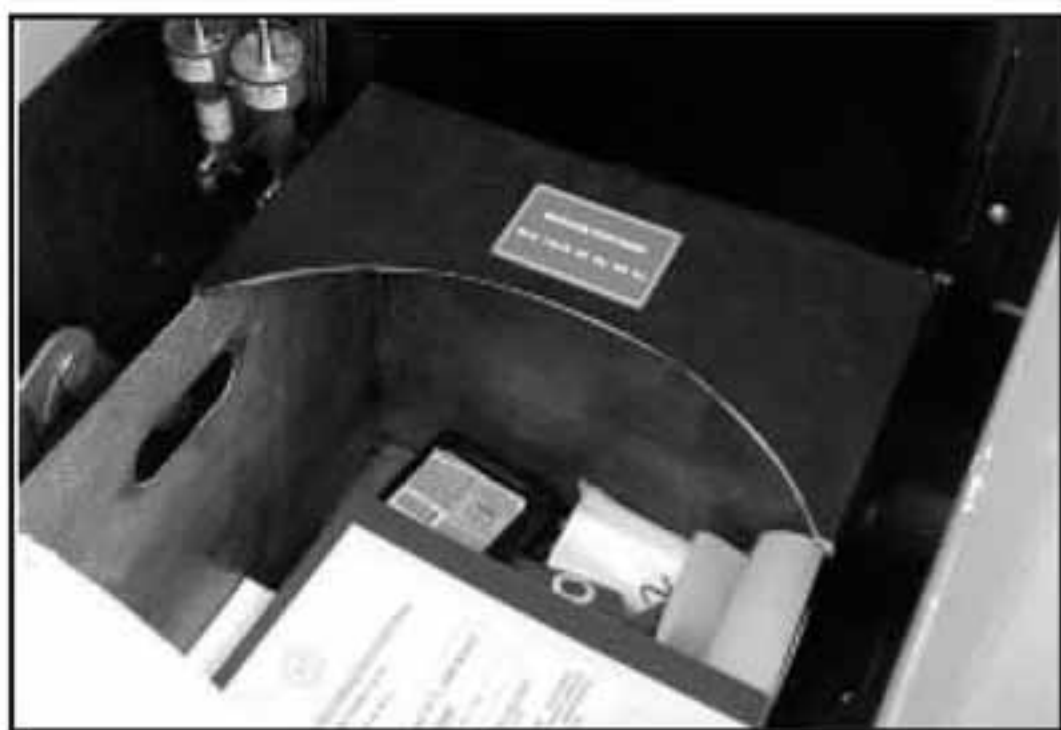
TWO SPACES - Underneath the aft seat is space for 66 pounds of luggage and aft of the seat is room for 33 pounds more. Fuel is also aft of the seat.
