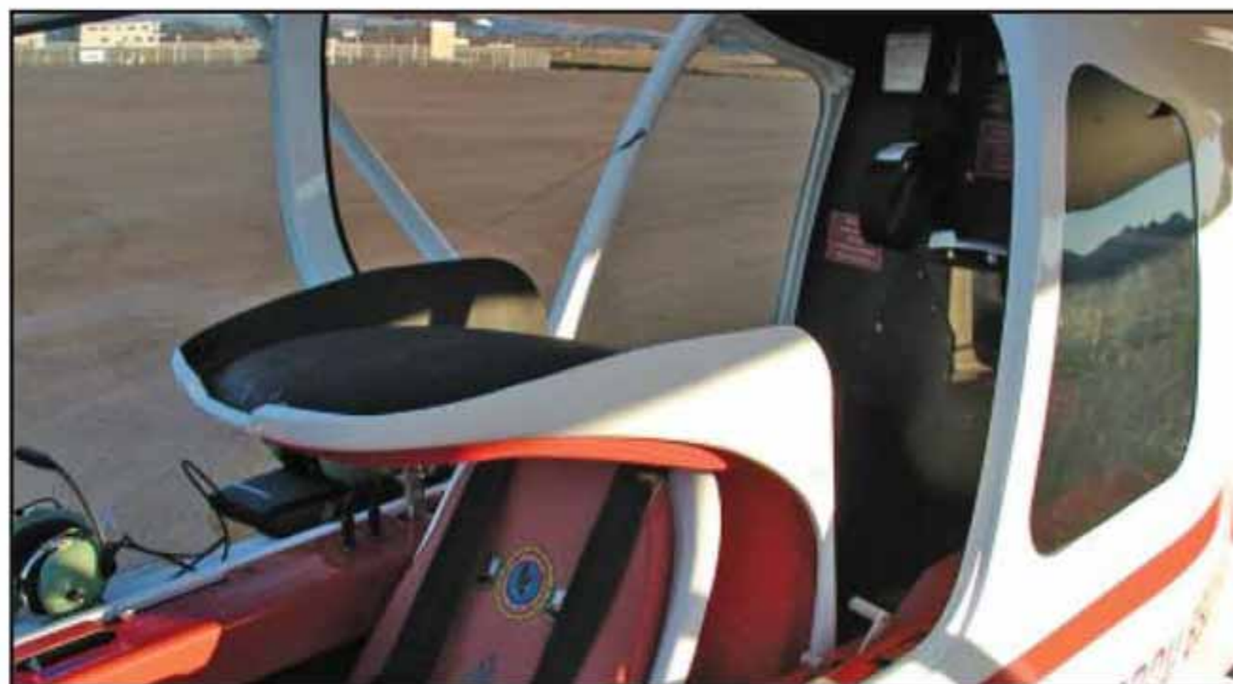
TILTED FORWARD - Initially you don't see any baggage area, but just tilt the aft seat forward to access two large areas.
